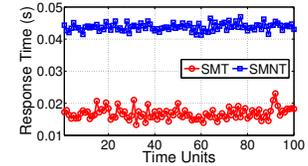
Fig. 14. Response time comparison between SMT and SMNT in fat-tree.
