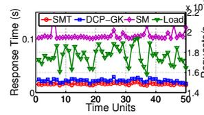
Fig. 5. In fat-tree, SM experiences about 7x controller response time compared with SMT.
