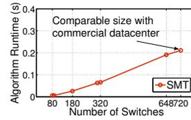
Fig. 13. Runtime of SMT under different topology scales.
