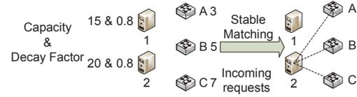
Fig. 2. The distance between switches and controllers is 1 hop. The stable matching solution yields an unbalanced situation that can be further improved by a transfer pair  $\{switch_B \rightarrow controller_1\}$  considering response time.
